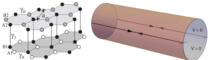
Figure 1 (left). AB stacked bilayer graphene. [3]  $\gamma_0 = 3.16$  eV,  $\gamma_1 = 0.381$  eV,  $a = 2.46$  Å. [4] Figure 2 (right). Cylindrical geometry, showing the two conducting channels where counterpropagating modes are localized.
