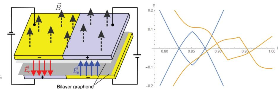
Figure 8 (left). Bilayer graphene with an electric field that changes sign at an interface and a uniform magnetic field. [5] Both fields are perpendicular to the plane of the bilayer. Figure 9 (right). Energy dispersion of the edge states at  $V_0 = 0.3$  for  $B = 0$  (blue) and  $B = 24$  (orange), showing the shifting K point.
